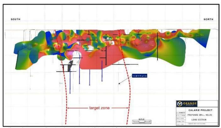
Figure 3- Long section showing planned drill holes at Calarie
