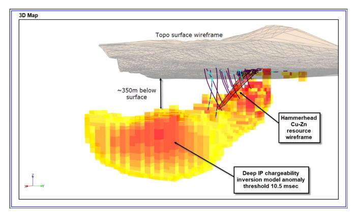
Figure 3 – IP Chargeability – Hammerhead Resource (Resource Potentials 2018)
